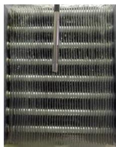
**Figure 3: Ice accumulated in the exchanger at 105 min (left) / Ice accumulated after pause at 108 min (right) for test B1.**
