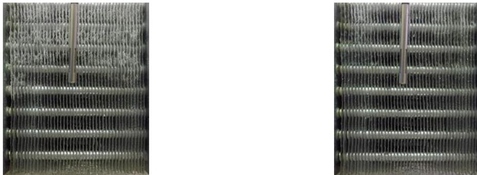
**Figure 6: Ice accumulated in the exchanger at 92 min, before interruption (left) and ice accumulated at 95 min, after the interruption (right).**
